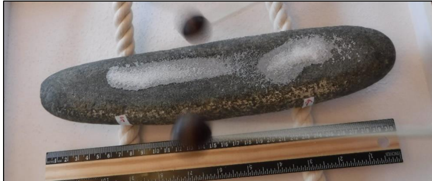
Notice how the salt is beginning to separate and migrate toward the nodes.
