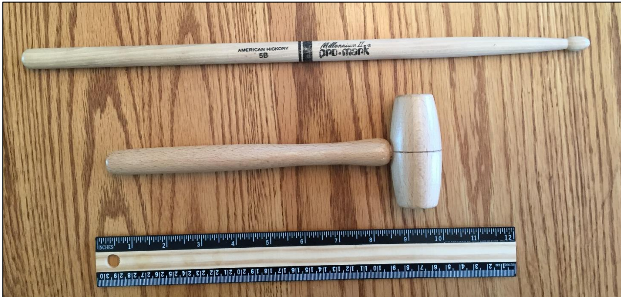
Figure 118. Drumstick and mallet made of wood; top – hickory drumstick used as a mallet, and bottom – boxwood mallet.
