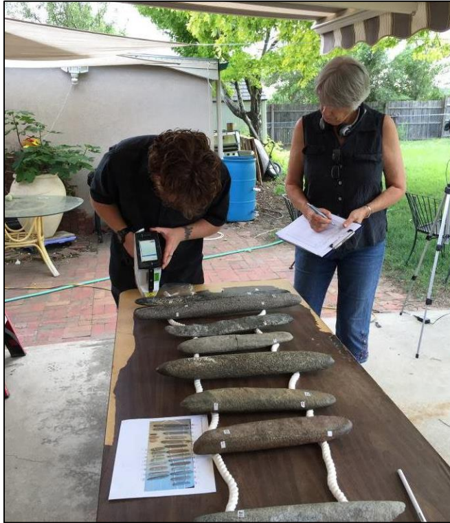
Figure 98. Linda Scott Cummings, PRI, and her assistant taking initial XRF readings to determine the chemical make-up of the lithophones.
